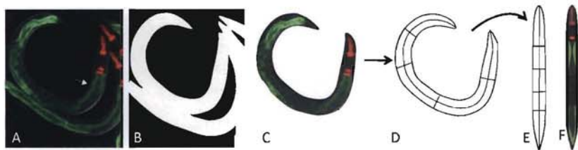
Figure C.8: Worm straightening (schematic). A: Original fluorescent image. B: Foreground/background segmentation of corresponding brightfield image. C: Single worm from fluorescence image. D: Medial axis and cross sections, straightened in E and re-sampled to F.
