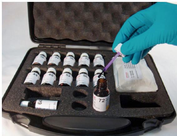
Figure 9.4 Set of dyne test liquids containing 12 fluid bottles ranging from 30 to 72 dynes/cm
