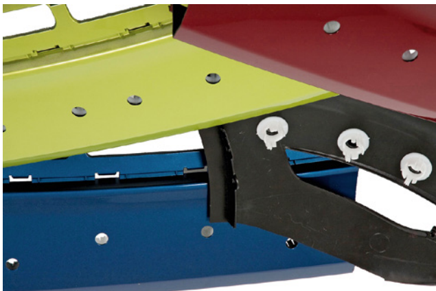
Figure 5.25 Painted automotive rocker panels having assembly locators mounted using the Soniqtwist® torsional ultrasonic machine
