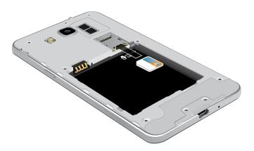
Carefully slide the SIM card into the SIM card slot.
