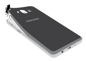
2. Lift the cover up and to the right of the device.
