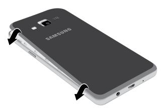
2. Press along the edge of the back cover until you have a secure seal.
