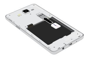
**Caution**: If the SIM card is not inserted correctly, the device cannot detect it. Reorient the SIM card and place it back into the slot if it is not detected.
