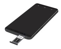
Slide the SIM card/Memory card tray back into the slot.  Carefully slide the SIM card into the SIM card slot. Make sure that the card's gold contacts face down into the device and that the card is positioned as shown.
