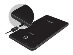
Insert the USB cable into the USB charger/ Accessory port.
