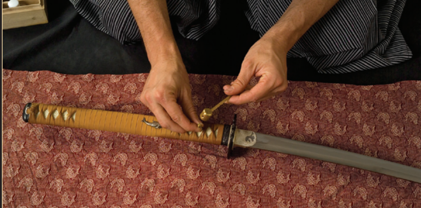
THE MAINTENANCE: The mekugi (pins) are driven out using a mekugi hammer. Once they're removed, the handle can be separated from the blade.
