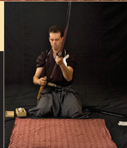
THE MAINTENANCE: The mekugi (pins) are driven out using a mekugi hammer. Once they're removed, the handle can be separated from the blade.
