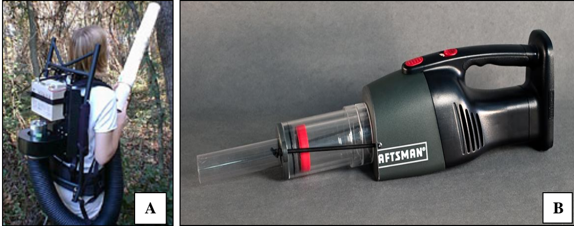
Fig. 4-1. Mechanical and oral aspirators. A. Backpack mechanical aspirator (John W. Hock Co.) B. Hand-held mechanical aspirator (BioQuip).
