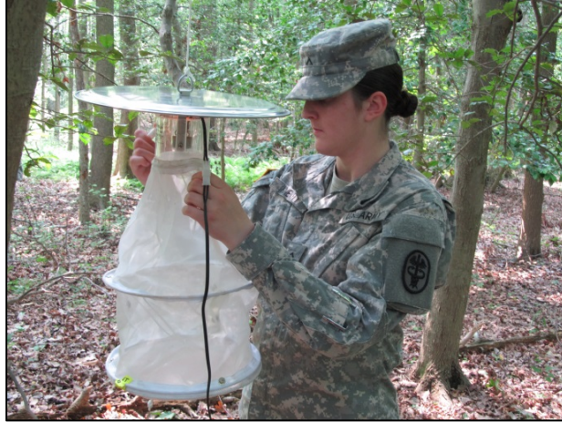
Fig. 4-4. Solid State Army Miniature (SSAM) trap.
