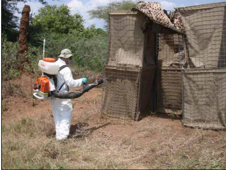
Fig. 6-1. Treating HESCO® units with Pestabs residual \lambda -cyhalothrin using a Stihl SR 450 backpack sprayer at an experimental plot in the Rift Valley, Kenya. Photo: Seth Britch, USDA.
