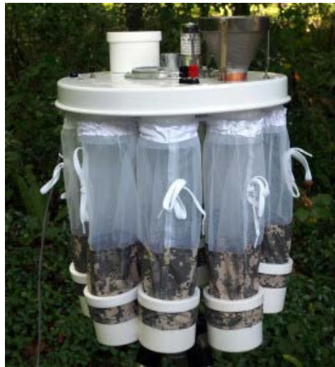
Fig. 4-5. Collection Bottle Rotator (CBR) trap. Photo: John W. Hock Company.
