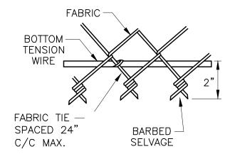
METHOD OF TYING FABRIC TO TENSION WIRES
