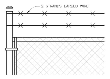
BARBED WIRE — 2 STRANDS, 12 1/2 GAUGE WIRE WITH 14 GAUGE 4 POINT BARBS SPACED APPROXIMATELY 6 INCHES APART. ALL WIRE SHALL BE ALUMINUM COATED WITH A MINIMUM COATING OF 0.25 OUNCES PER SQUARE FOOT OF SURFACE AREA.
