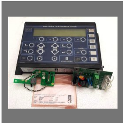
KONGSBERG 8100255 LOCAL OPERATOR PANEL LOS
