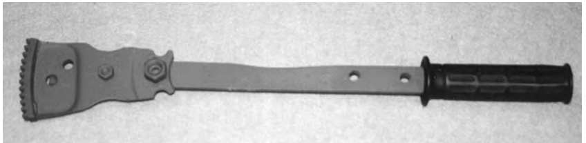
Homemade tool cut from an old flex plate to lock the engine to torque either the flywheel or harmonic balancer retaining bolt when the cylinder head is on.
