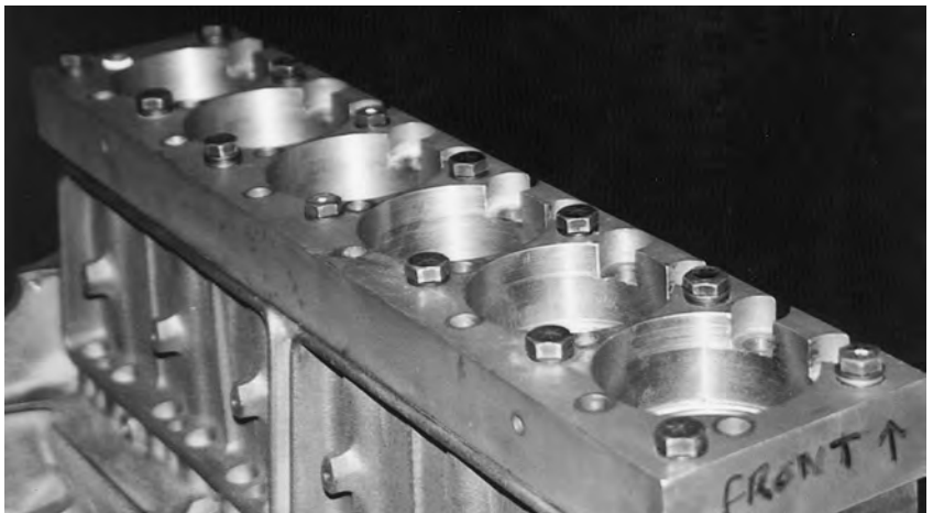
Torque plate—shown as dual pattern for stock bolt pattern and also for hybrid head (Chevy V8).
