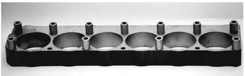
Traditional torque plate by Yother. This plate, when bolted to the block, simulates the effect on the bore when the cylinder head is bolted on. Note spacers added to top of plate. This allows the use of stock-length bolt or stud, which simplifies using this plate. A thick plate is necessary to duplicate stresses created by the cylinder head.
