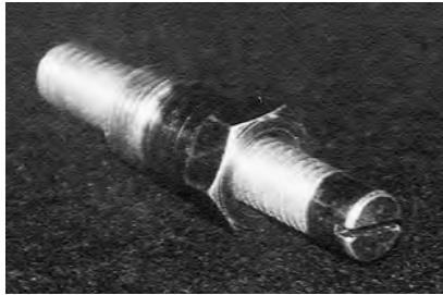
Positive stop when head is on the engine (screws into the spark plug hole).
