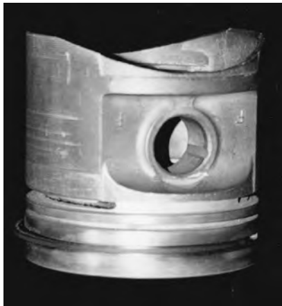
Homemade piston ring squaring tool, simply an old piston with the compression ring in place. Invert the piston, place ring in the cylinder and push down until the compression ring on the piston stops against the block. Remove the piston and measure the ring gap.
