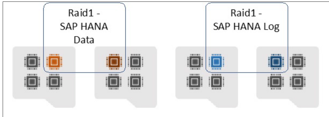
Figure 3-16 RAID 1 storage volumes for SAP HANA data and logs by using NVMe adapters
