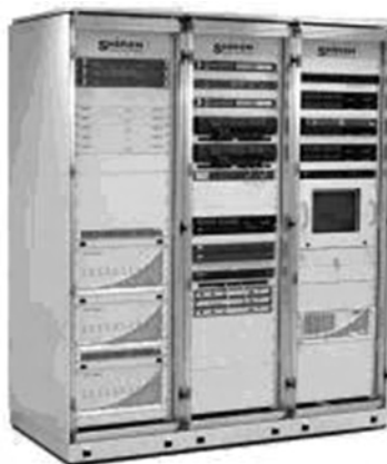
Gambar 2.13 Hub station VSAT
