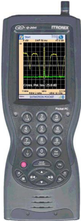
Integrasys' SATMOTION POCKET (US patent pending 10/408710) is a simple and low-cost tool for VSAT installers.
