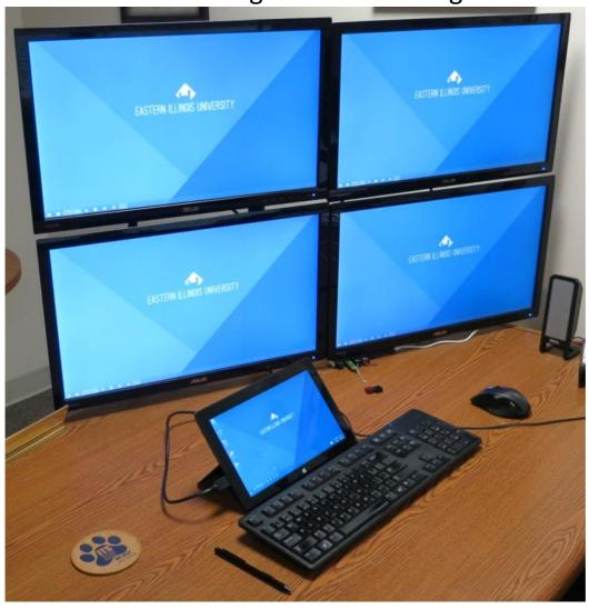
This is a Surface Pro 2 connected into a Pluggable docking station using just the USB 3.0 port. This solution supports 4 external monitors and keyboard using just one USB cable from the Surface Pro 2!!!
