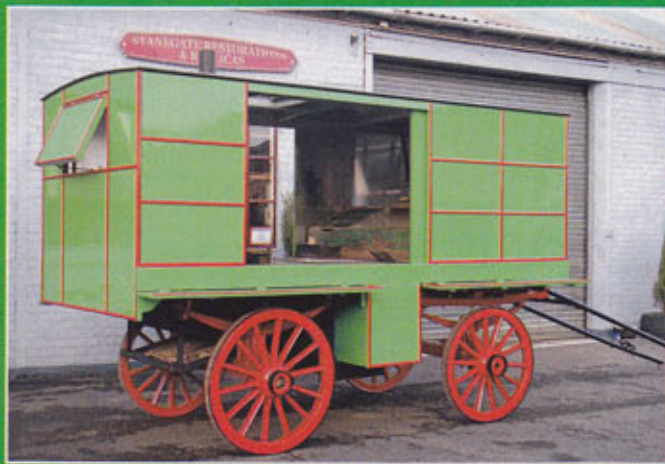
The chip van is almost finished, with the beading highlighted in red.
