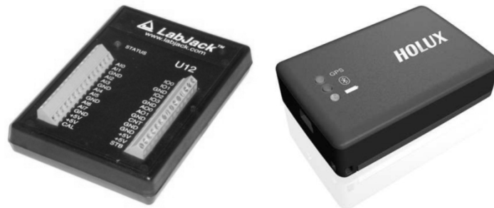
Fig. 2. Left GPS device Holux M-1000C and measuring card right LabJack U12
