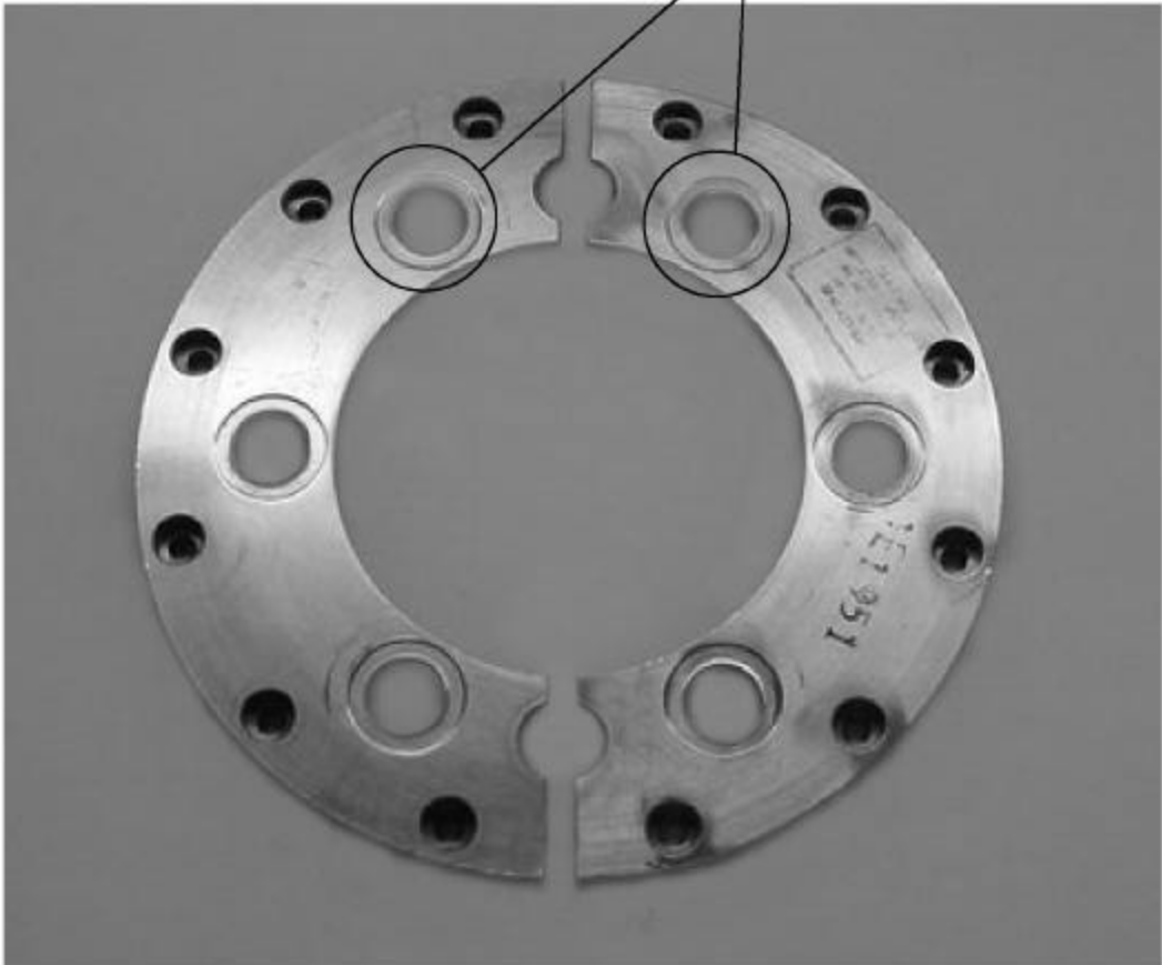
DAMAGED MOUNTING PLATE
