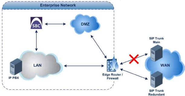
Figure 3-1: SIP Trunk Redundancy Example Scenario
