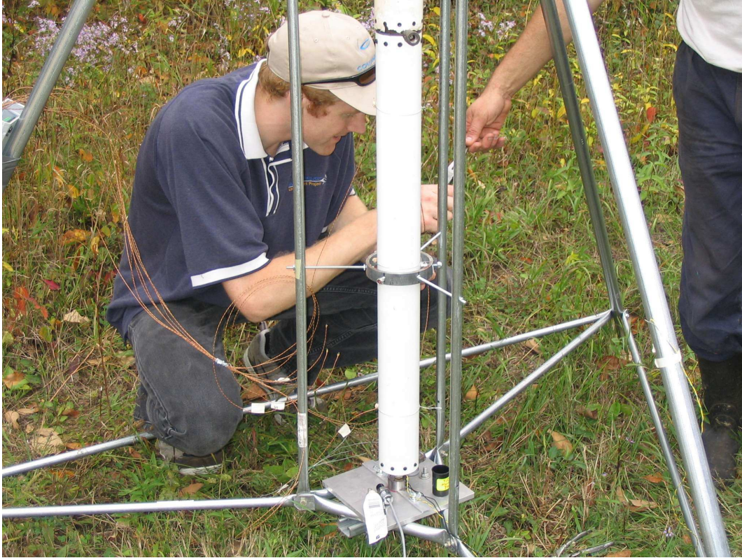
Photo 5 – Daniel mounting thermocouples on motor
