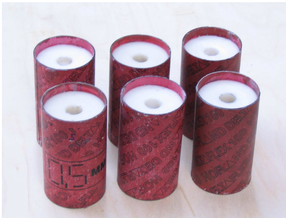
Photo 2 – Propellant grain segments prior to coating ends with ignition primer
