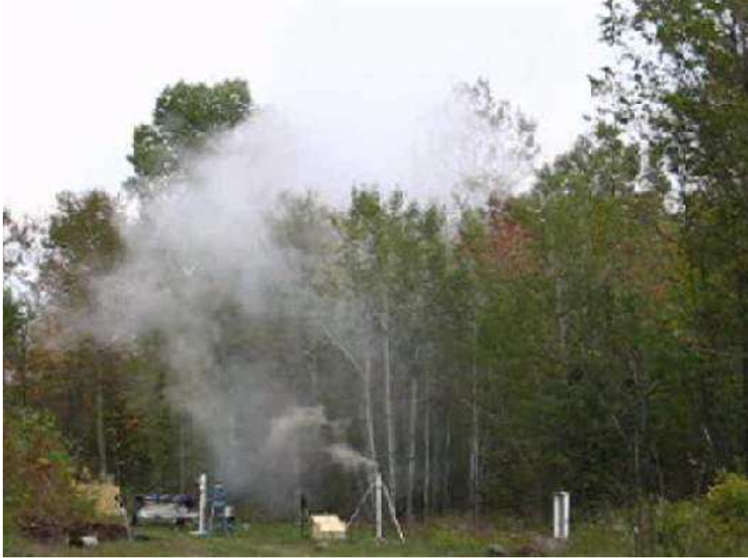
Photo 7 – Following burnout of 1 st phase, smoke issues from burning delay plug
