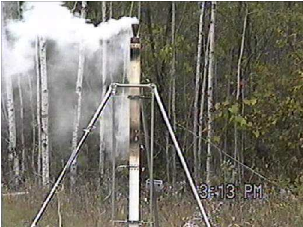
Photo 10 – Motor smoulders following burnout
