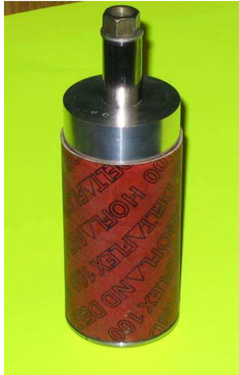
Photo 1 – Grain segment casting mould used for 1 st phase
