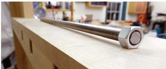
Bolt stretcher. I used Loctite Threadlocker Red 271 to permanently (I hope!) affix a nut to the end of my threaded rod. The break point for the thread locker was sufficiently high that I could really cinch things down. Use a torque wrench set lower than the break point of the ThreadLocker and you'll be fine.
