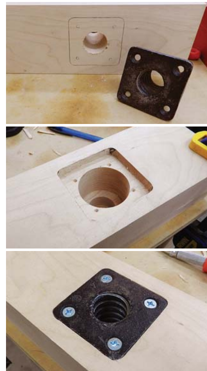
Shoulder vise screw. After drilling a clearance hole, use that to locate the plate of the screw hardware, and trace around it. After removing the waste to inset the plate, screw the plate in place.
