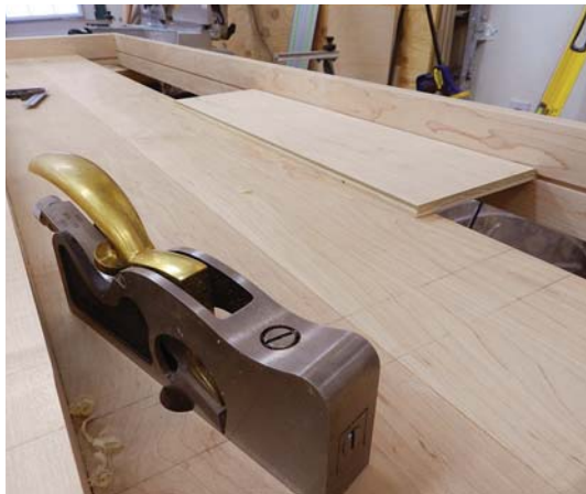
Test-fit. Use a scrap to test the fit of the tool tray bottom to its rabbet. Once you have it dialed in, you use a shoulder plane to fine-tune the joint.
