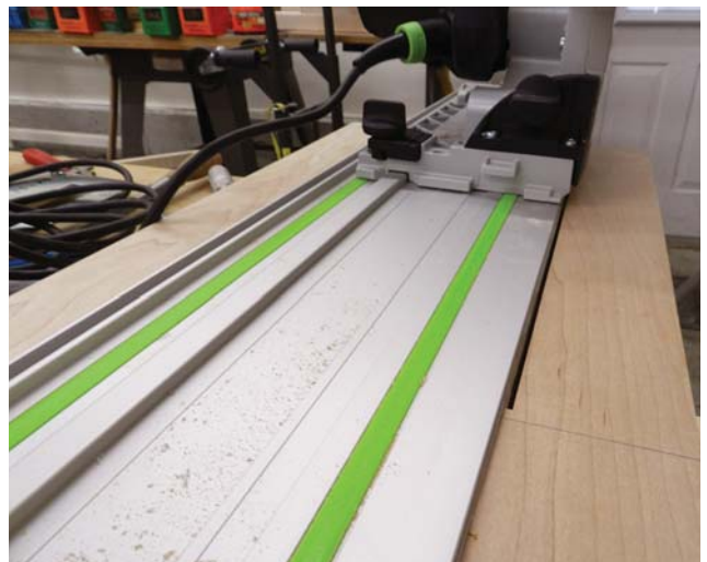
On track. A track saw or circular saw with a guide makes quick work of removing the waste where the tail vise goes.
