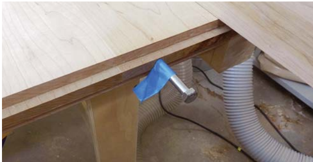
Know your depth. Test the hole depth with a bolt taped off at the max depth you expect it to reach, given the depth it will be into the end cap.
