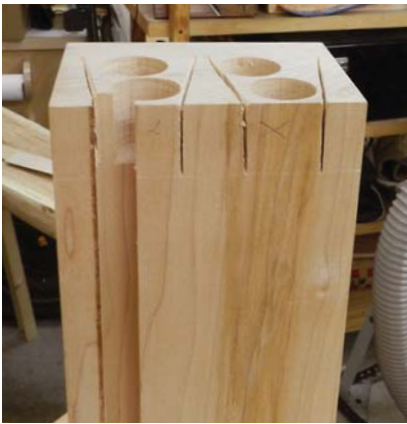
Pin layout. When laying out the half-blind dovetails on the rear skirt, make sure the groove for the tool tray falls in a socket, where it will be covered by a tail.
