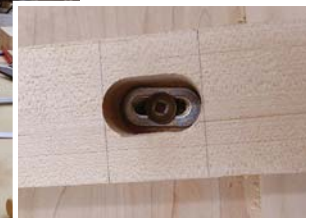
The view from below. Expansion washers and screws secure the filler blocks and allow for seasonal movement.
