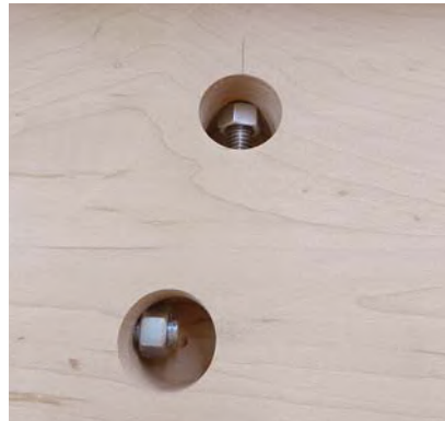
Access holes. The size of the holes on the underside of the bench doesn't really matter – they just need to be large enough to accommodate attaching and securing nuts and washers on the ends of the bolts.
