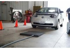
Researchers at Oak Ridge National Laboratory test a wireless power transfer charger on a fully electric vehicle. [US Department of Energy photo]
