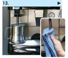
• Submerge steam wand into cold water once to rinse, then discard water. Wipe steam wand with a clean, damp cloth.
