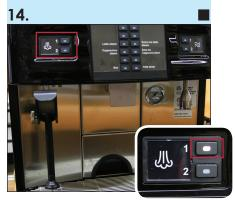
• After wiping off wand, point it toward drip tray and purge by pressing the button **1**.
