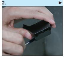
• Using small cleaning brush, brush the 2 holes, then wash, rinse and sanitize. Dry the coffee spout thoroughly with a clean, damp cloth.
