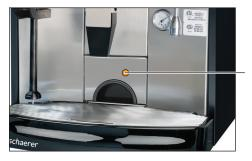
The grounds bin is located below and behind the coffee spout. It holds the used grounds which are disposed of after each espresso shot is brewed. The bin slides straight out from the machine and must be emptied periodically or when prompted on the display.
