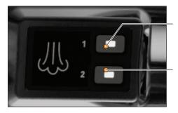
To purge the steam wand after each use, press purge button **1**. It will purge for two seconds and stop automatically. Or, press the button again to stop manually.
