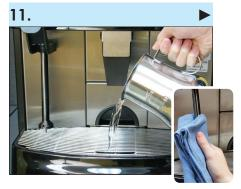
• After 5 minutes or when automated cleaning cycle is complete, empty pitcher into drip tray. Wipe steam wand with a thick, clean, damp cloth. **Be careful, wand will be very hot!**
