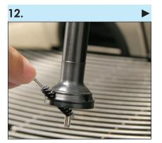
• Using small cleaning brush, brush the 4 side holes as well as base of the steam wand tip.
