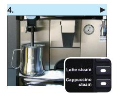
Submerge steam wand into steaming pitcher and press the LATTE STEAM button to heat solution. After steam wand shuts off automatically then let it soak for 5 minutes.
