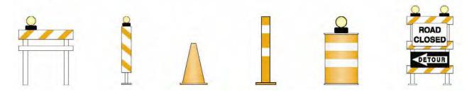
The diagonal stripes on the barricade or vertical panel guide the driver toward the direction to which traffic is to pass. Stripes sloping downward to the right mean the driver should bear to the right. Conversely, stripes sloping downward to the left mean bear to the left.
