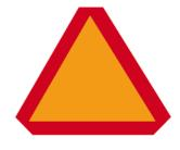
The emblem shall be a triangle of fluorescent yellow-orange color with a base of 14" and 14" in height. The triangle shall have a border with reflective red stripes one and three-quarters inches wide and shall be mounted in the center of the rear of the vehicle at a height of three to five feet above the roadway.
