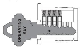
The operating key cannot be removed in the lockout position because the back two pins are unable to disengage from the key
