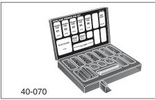
Contains finger pins, finger pin springs, sidebars, sidebar springs and plug holder (40-066).
