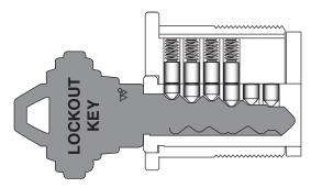
The last two notches in the key are removed allowing the key to exit the cylinder.
