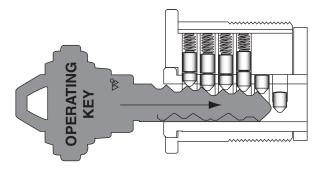
The operating key cannot enter the cylinder because the back two pins are not able to settle into their bitting spaces on the key.
