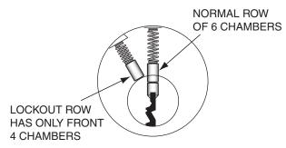
When the plug is in its standard operating position all keys will operate the lock. To temporarily disable to regular operating keys, the plug can be turned with the special key to align the bottom pins with the lockout row of pins.
