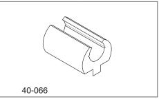
Has grooves for Primus sidebar. Included in 40-070 finger pin kit.
