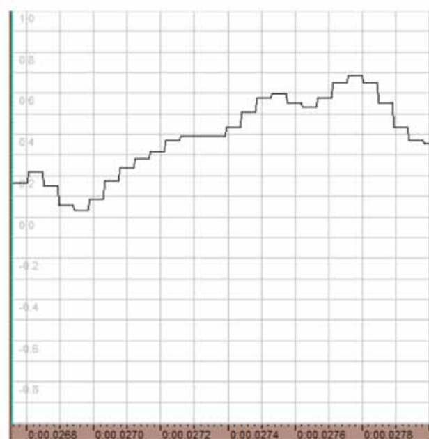
Figure 3.7: Zoom view of the digitised waveform
