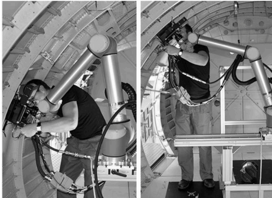
Figure 7: Human-Robot-Collaboration in Aircraft Assembly [19]
