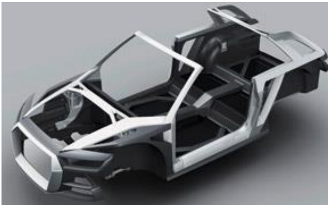
Multimaterial-Space-Frame Audi Crosslane Coupé [Quelle: lightweightdesign]
