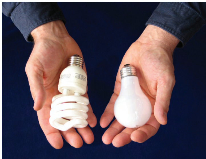
Figure 2-16 Two widely used technologies waste enormous amounts of energy. In an incandescent lightbulb (right), about 95% of the electrical energy flowing into it becomes heat; just 5% becomes light. By comparison, in a compact fluorescent bulb (left) with the same brightness, about 20% of the energy input becomes light. In the internal combustion engine (right photo) found in most motor vehicles, about 87% of the chemical energy provided in its gasoline fuel flows into the environment as low-quality heat. (Data from U.S. Department of Energy and Amory Lovins; see his Guest Essay at CengageNOW.)
