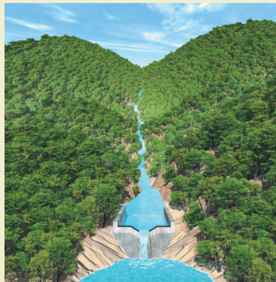
Figure 2-1 This controlled field experiment measured the effects of deforestation on the loss of water and soil nutrients from a forest. V-notched dams were built at the bottoms of two forested valleys so that all water and nutrients flowing from each valley could be collected and measured for volume and mineral content. These measurements were recorded for the forested valley (left), which acted as the control site, and for the other valley, which acted as the experimental site (right). Then all the trees in the experimental valley were cut and, for 3 years, the flows of water and soil nutrients from both valleys were measured and compared.
