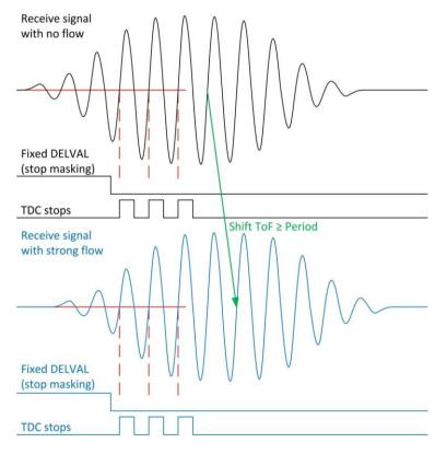
Figure 4-10: Typical error by high fluid dynamics
