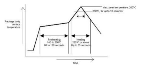
Figure 2-9 Soldering profile
