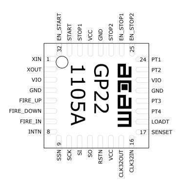
Figure 2-6 TDC-GP22 Pinout
