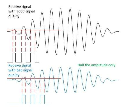
Figure 4-11: Wrong measurement due to signal damping
