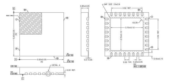
Figure 2-7 QFN-32 package outline, 5 x 5 x 0.9 mm³, 0.5 mm lead pitch
