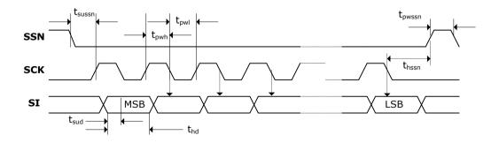
Figure 2-2 SPI Write
