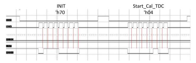
Figure 3-1: Sample scope picture for sequence INIT 'h70 and Start Cal TDC = 'h04
