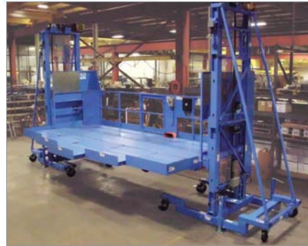
Dual Mast Work Platform
