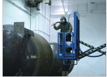
Multi-Axis Blast Booth Lift
