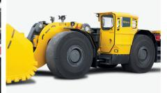
Through the redesign of a lower profile boom system we offer the best operator visibility in its class and Scooptram ST14 is equipped with extra spotlights on fenders making it easier and safer to load trucks.
