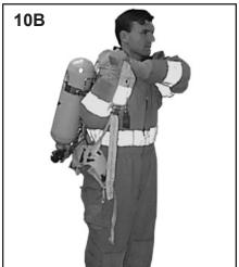
c) While leaning slightly forward, slide unit down back and pull on shoulder adjusting straps. Ensure that the shoulder pads fall into place on the shoulders.
