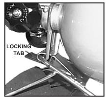
FIGURE 19A FIGURE 19B Locking tab mechanisms
