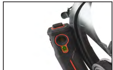
FIGURE 27 GREEN POWER LIGHT
