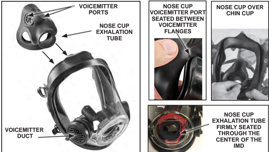
FIGURE 19 INSTALLING THE NOSE CUP
