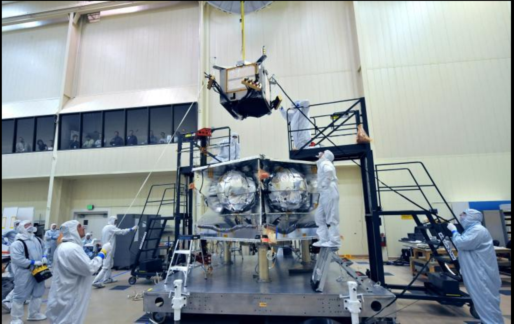
Moving the Titanium radiation vault (with some avionics already installed) over to the propulsion module
