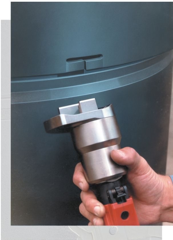
RL-4 anti-rotation tab and hand-held locking tool
