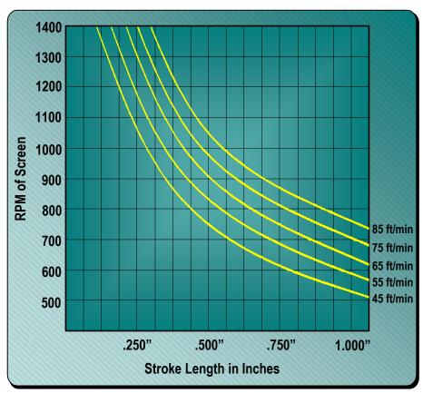
Figure 24, Chart C - Conveying Velocity at 50° Timing Angle Flat Screens
