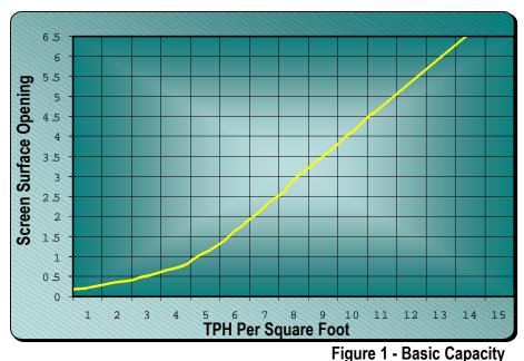
capacity of a deck is "**A**" multiplied by the area of the deck in square feet. This is the final result of the multiplication of all the screen factors.
