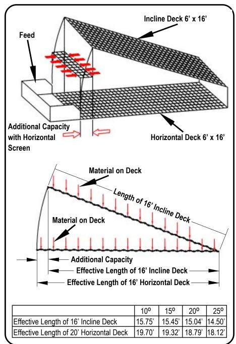
Figure 2 - Deck Comparison, Incline to Flat
