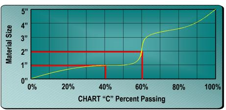
Figure 21, Chart C - Material Distribution Curve with Reduced 2" Near Size
