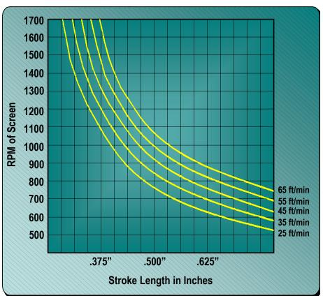
Figure 23, Chart C - Conveying Velocity at 10<sup>o</sup> Incline Incline Screen with Circular Stroke
