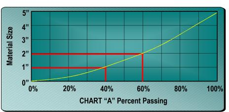
Figure 21, Chart A - Normal Material Distribution Curve
