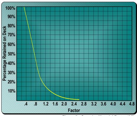
Figure 5 shows the percent retained as a measure of oversize material. The related oversize factor is picked off the intersection of percent retained and the curve. For example, 25% oversize generates a **"V"** factor of 1.0.
