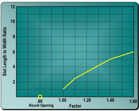
openings have a 0.8 slot factor. Any difference in capacity based on the direction of the slots being either with, or across, the flow of material is not taken into account. When calculating screen capacity blinding is not directly considered. Spring loaded wirecloth (Z wire) does not increase the slot factor over that of standard slotted wire. Spring-loaded wirecloth does help prevent blinding, however, and maintains open area. Determine slot factor based on Figure 7.
