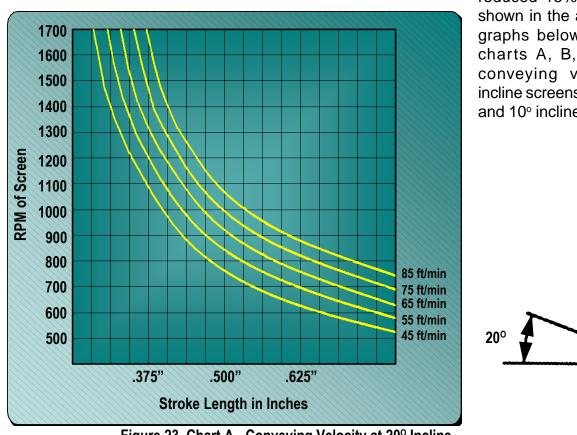
reduced 15% from what is shown in the accompanying graphs below. Figure 23, charts A, B, C, illustrate conveying velocities for incline screens set at 20°, 15° and 10° inclines.
