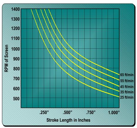
Figure 24, Chart G - Conveying Velocity at 30° Timing Angle Flat Screens
