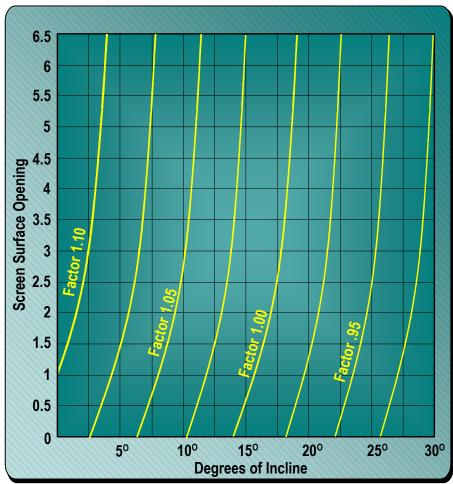
Figure 3 - Incline Angle Factor "S"
