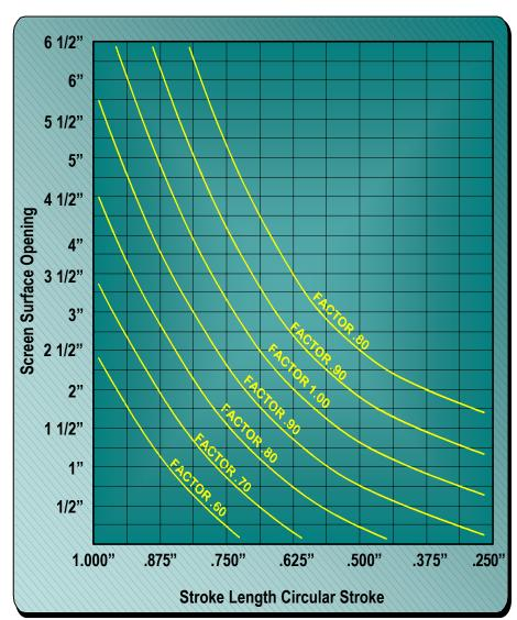
Figure 17 - Stroke Length Factor for Incline Screens
