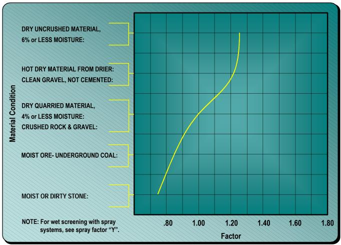
Figure 8 - Material Condition "K"
