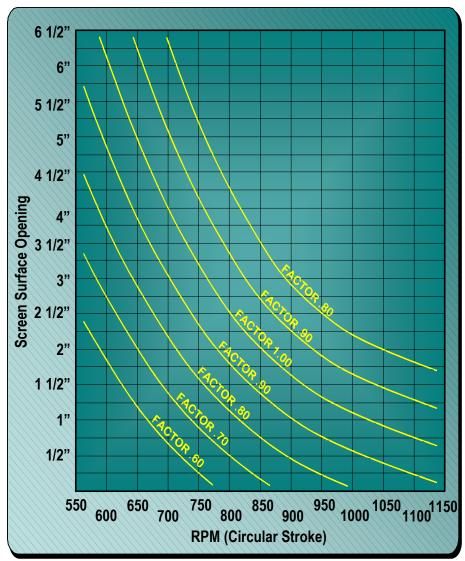
Figure 20 - "RPM" Factor for Incline Screens
