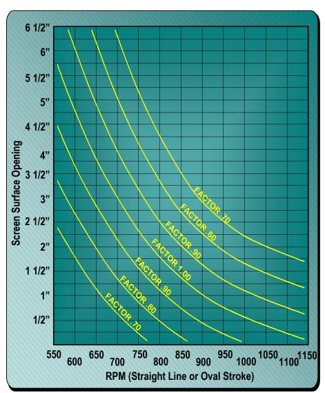
Figure 19 - "RPM" Factor for Flat or Horizontal Screens
