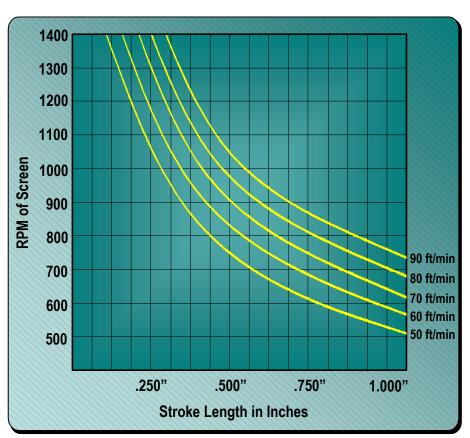
Figure 24, Chart B - Conveying Velocity at 55° Timing Angle Flat Screens
