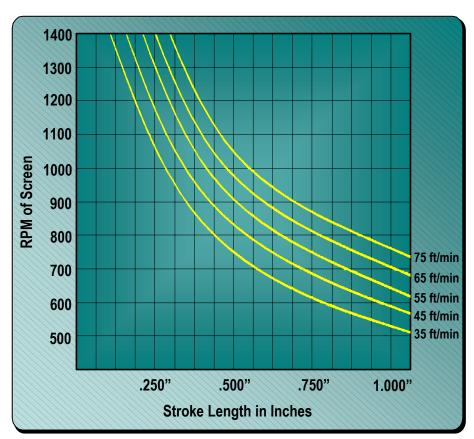
**NOTE:** Screening media and shape of material to be screened greatly effect conveying velocity.
