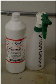
Spray the solution onto the screen and let it sit for 1-2 minutes (not more). Fix
