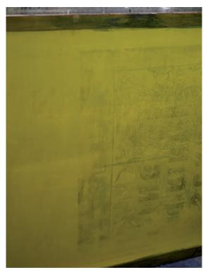
• Lastly, spray degreaser onto both sides of screen and wipe it with a clean cloth. Then wash out again, and place it back into the rack.
