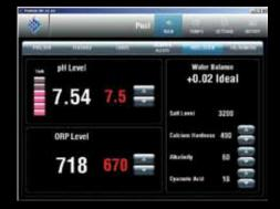
The IntelliChem® chemical controller interface enables customers to monitor their pH and sanitizing levels from their controller, rather than visiting the equipment pad. Compatible with Pentair's IntelliChlor salt chlorine generators, liquid feed pumps and CO<sub>2</sub> systems.
