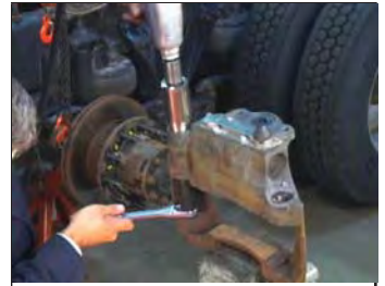
FIGURE 71 - REMOVE THE LONG GUIDE PIN
