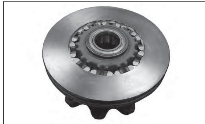
FIGURE 90 - INTERMEDIATE ELEMENTS (SPACERS) INSTALLED
