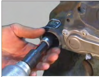
FIGURE 67 - REMOVE THE CALIPER BOLTS
