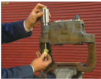
FIGURE 70 - INSTALL THE REMOVAL TOOL
