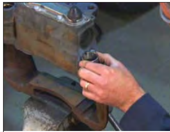
FIGURE 78 - POSITION THE NEW BUSHING
