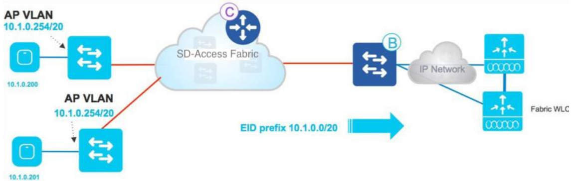
Figure 36. Access points in SD-Access Wireless
