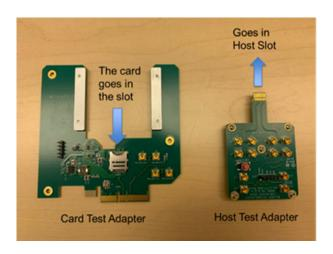
Figure 14 microSD Card and Host test adapters
