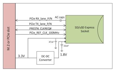
Figure 5 M.2/PCIe to SD7.x Adapter
