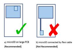
Figure 17 Recommended PCB high level design concepts
