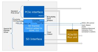
Figure 7 Block Diagram of SD Express Host with new Control lines
