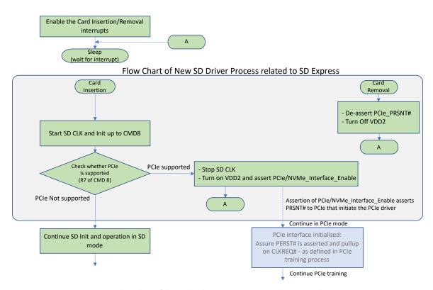
Figure 13 Flow Chart of the updated SD Drivers Operation during Initialization
