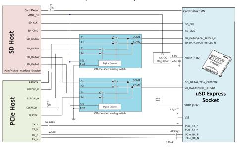
Figure 8 A Practical Example of Mux/De-Mux circuit
