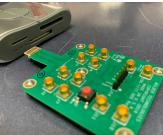
Figure 16 microSD Express and SD Express Host Test Adapters may be inserted to related SD Express hosts
