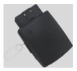
Place the micro-SIM card on the tray with the gold-colored contacts facing down and slide the tray back into place.
