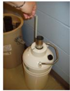
Step: 3 Load the dry shipper with cryovials you have stored at -80°C
