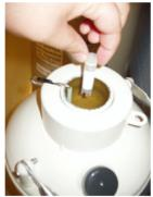
Step 4: Place cap back on the dry shipper and secure with a cable tie (zip tie) for transport.
