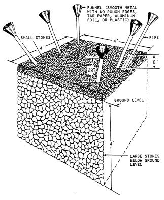
Figure 10-56.—Urinal pipes and soakage pit.
