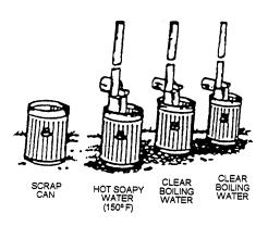
Figure 10-57.—Immersion heaters for mess kit washing setup.
