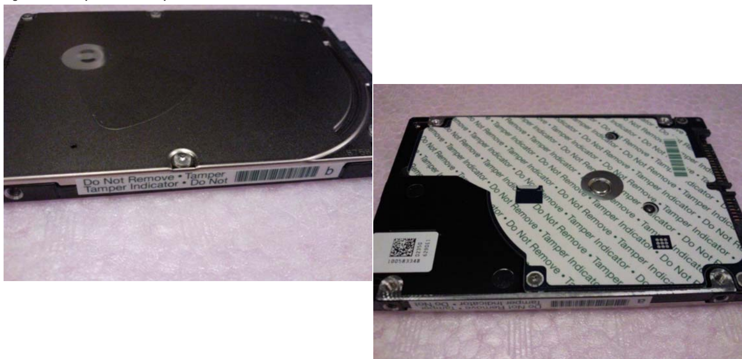
Figure 5 Example of FIPS tamper evidence labels.
