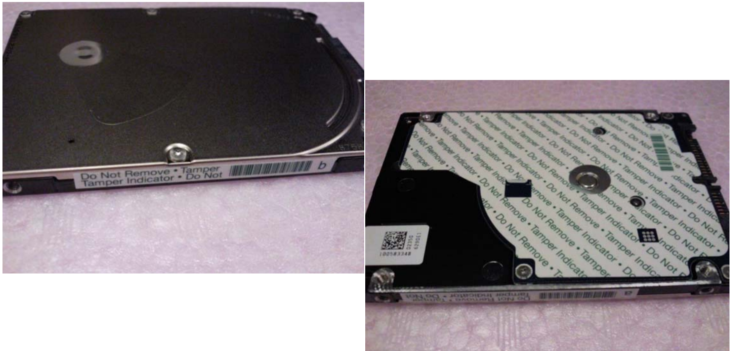
Figure 5 Example of FIPS tamper evidence labels.
