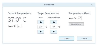
Figure 12. Edit temperature settings (Tray Heater dialog box)
