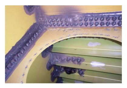
Figure 2. Sealant covering fasteners in the center wing tank
