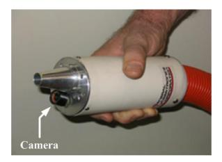
Figure 7. GLC confined space tool for laser coating removal
