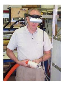
Figure 6. Operator uses video display if line-of-sight obstructions exist
