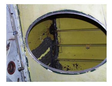
Figure 3. Example of results of mechanical (scraping) to remove sealant
