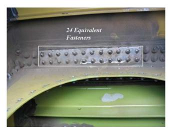
*Figure 9.* Sealant completely removed from a larger area (same area as shown in Figure 2).
