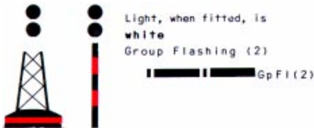
Figure 5-30.—IALA Maritime Buoyage System isolated danger marks.
